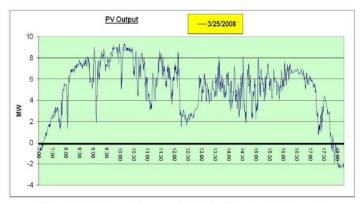
Figure 2.12: PV Plant output on a partly-cloudy day (Sampling time 10 seconds)
